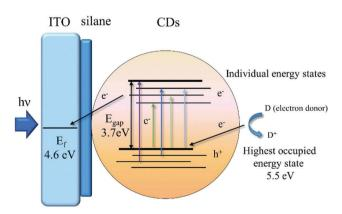
Fig. 4 The mechanism of photoelectric conversion of CDs.
