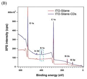
**Fig. 2** (A) Scheme of CDs binding onto ITO *via* a reaction with 3-glycidoxypropyldimethoxymethylsilane; (B) XPS full scan spectrum of the ITO-silane and ITO-silane-CDs.
