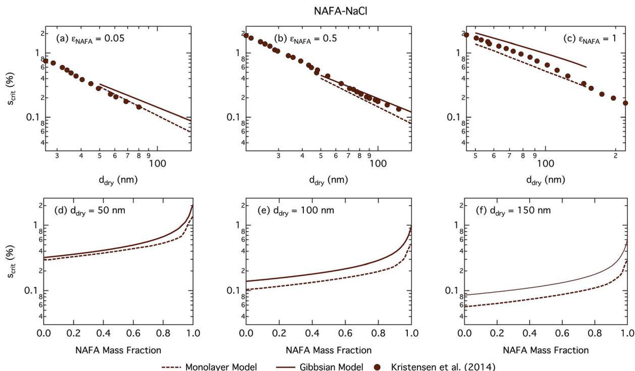
**Fig. 8** Critical supersaturations calculated with the monolayer and Gibbs models as a function of dry particle size for NAFA mass fractions (a) 0.05; (b) 0.5; (c) 1 and as a function of NAFA mass fraction for dry particle sizes (d) 50 nm; (e) 100 nm; and (f) 150 nm. Measured critical supersaturations as a function of dry particle size from Kristensen *et al.*<sup>14</sup> are also shown in panels (a)–(c). The measurements in panel (a) are for pure NaCl and are shown for comparison.
