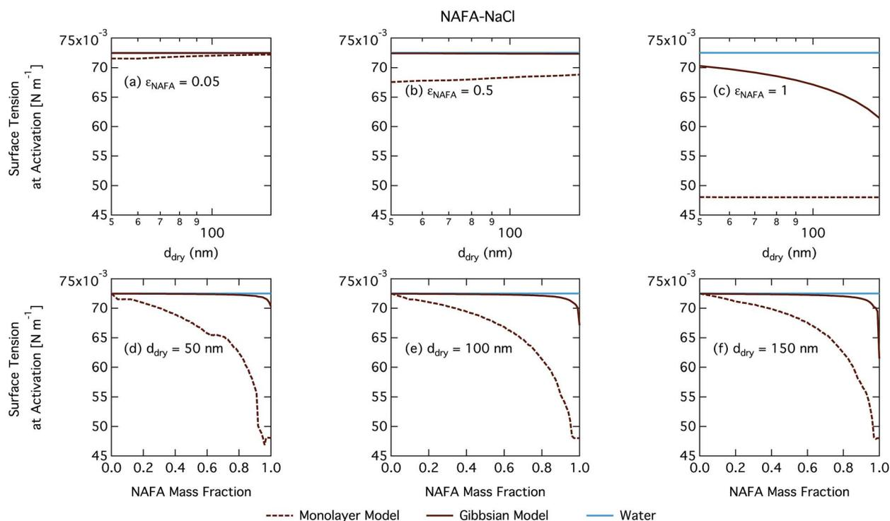
**Fig. 9** Surface tension at activation calculated with the monolayer and Gibbs models as a function of dry particle size for NAFA mass fractions (a) 0.05; (b) 0.5; (c) 1 and as a function of NAFA mass fraction for dry particle sizes (d) 50 nm; (e) 100 nm; and (f) 150 nm.
