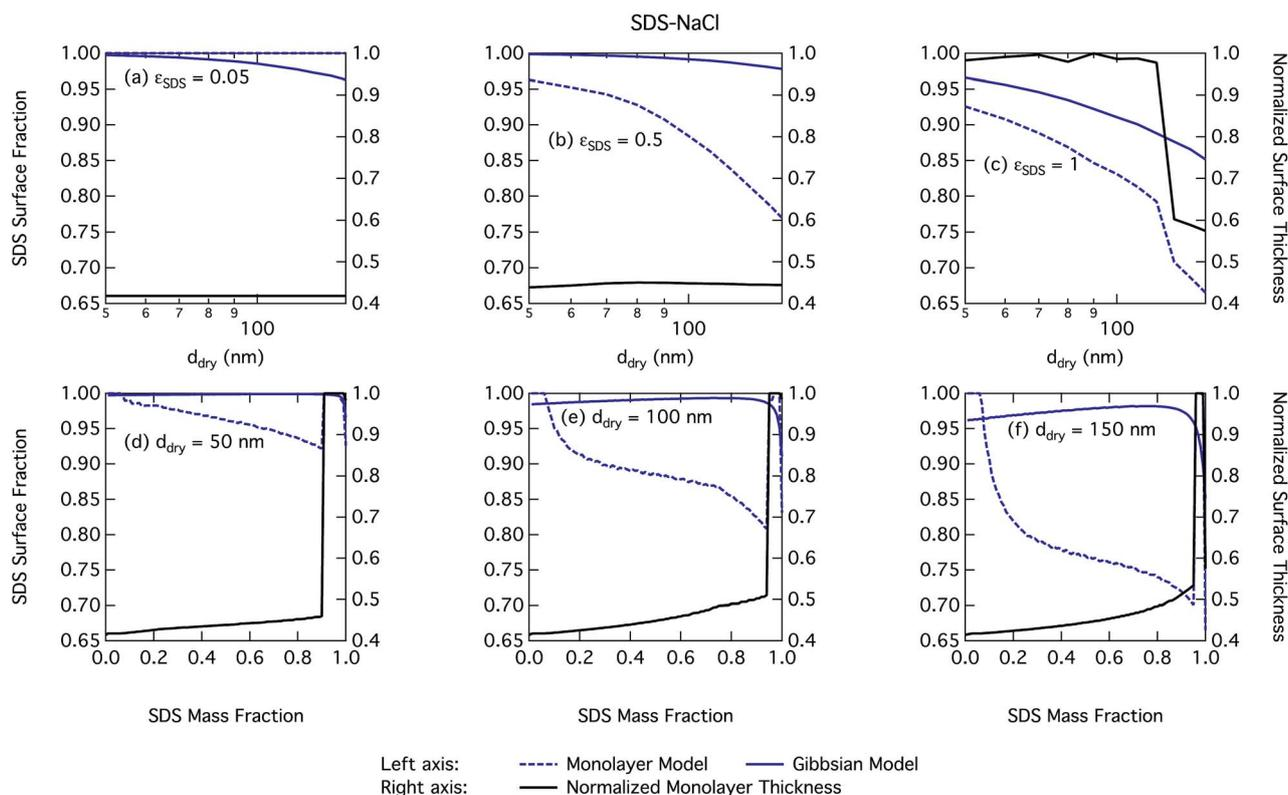
Fig. 7 Droplet SDS surface fraction on the left axes calculated with the monolayer and Gibbs models and surface thickness from the monolayer model normalized to the thickness of one SDS monolayer on the right axes as a function of dry particle size for SDS mass fractions (a) 0.05; (b) 0.5; (c) 1 and as a function of SDS mass fraction for dry particle sizes (d) 50 nm; (e) 100 nm; and (f) 150 nm.
