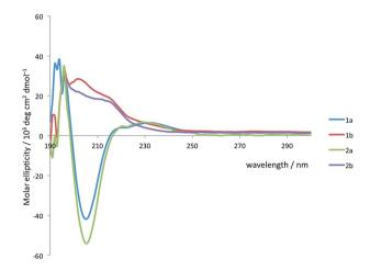
Fig. 4 CD spectra of  ${\bf 1a}$  and  ${\bf b}$  and  ${\bf 2a}$  and  ${\bf b}$  recorded at  $2.4\times 10^{-4}$  M in MeOH at 20 °C.
