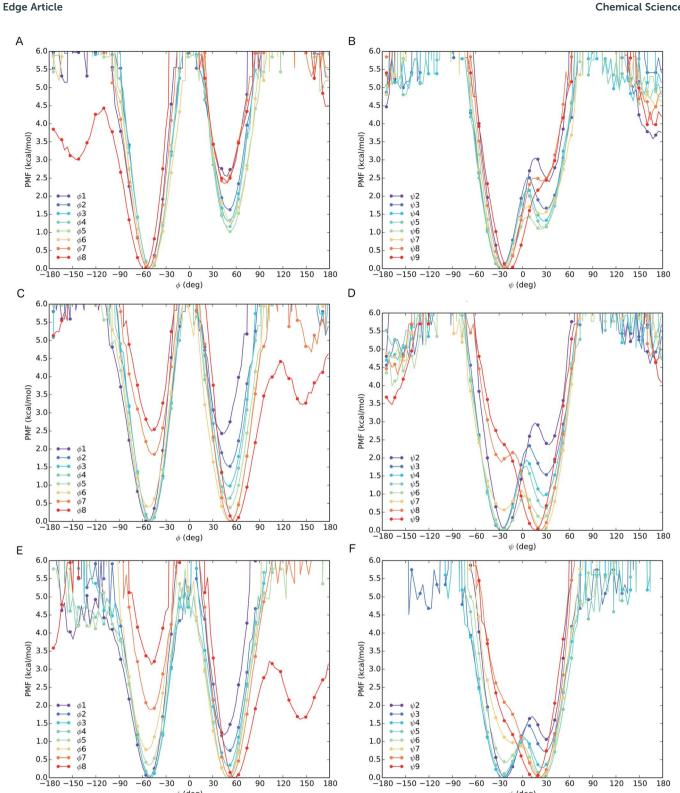
Fig. 7 PMF as a function of  $\varphi$  (A) and  $\psi$  (B) dihedrals for oligomer **1a** and of  $\varphi$  (C) and  $\psi$  (D) dihedrals for oligomer **1b** from REMD simulations in implicit solvent. PMF as a function of  $\varphi$  (E) and  $\psi$  (F) dihedrals for oligomer 1b from REMD simulation in explicit MeOH.
