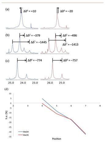
Fig. 12 Portions of the <sup>13</sup>C NMR spectra recorded at 23 °C in MeOH (blue, left) and MeCN (red, right), with  $\Delta\delta$  values in ppb, of (a) **6a**, (b) **6b** and (c) **6c**. (d) Plot of h.e., calculated from chemical shift difference  $\Delta\delta$ in the <sup>13</sup>C NMR spectrum recorded in methanol (blue) and acetonitrile (red), against the position in the chain, showing a change from an M to a P screw-sense at around Aib4. (Negative h.e. indicates an M screwsense.)
