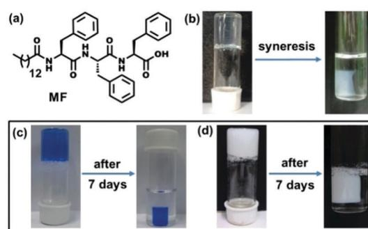
**Fig. 1** (a) The chemical structure of the amphiphile **MF**. (b) Image showing transparent fresh hydrogel obtained from **MF** (at 1.5 mM concentration) and 7 day aged opaque gel upon syneresis. (c) Photographs of the dye (Brilliant blue) containing hydrogel before and after syneresis. (d) Photographs of Pb<sup>2+</sup> ion containing hydrogel before and after syneresis.
