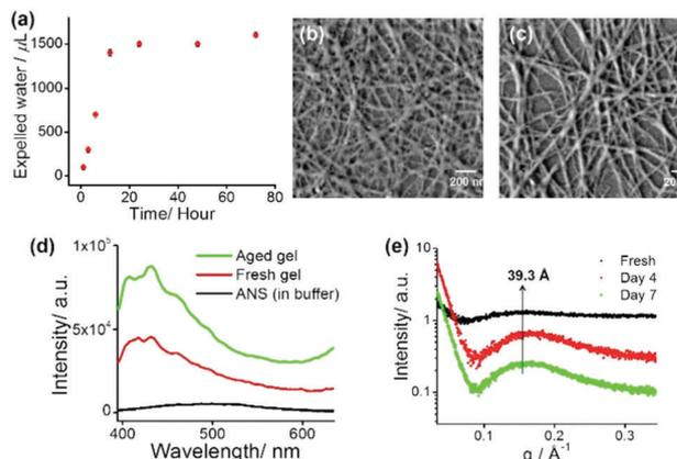
Fig. 2 (a) Amount of expelled water with time showing the dynamic shrinkage behaviour of the hydrogel obtained from **MF**. Image showing FE-SEM images obtained (b) immediately after gel formation and (c) after 7 days of syneresis. (d) ANS binding fluorescence assay of the gel showing an increase in fluorescence during syneresis. (e) SAXS data obtained from the xerogels (obtained from freshly prepared, 4 day and 7 day aged gels).
