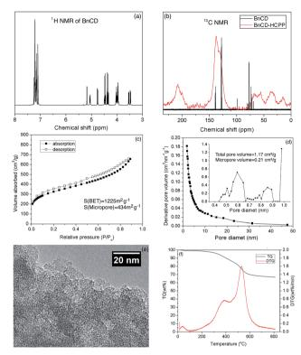
Fig. 1 (a)  $^1$ H NMR spectrum of BnCD, (b)  $^{13}$ C NMR of BnCD and solid-state  $^{13}$ C NMR of BnCD-HCPP (spinning at 7 K), (c) N $_2$  adsorption—desorption isotherms of BnCD-HCPP measured at 77 K (the polymer was pretreated at 170  $^{\circ}$ C under nitrogen flow for 2 h), (d) pore size distribution of BnCD-HCPP, (e) transmission electron microscope image of BnCD-HCPP, and (f) thermogravimetry and differential thermogravimetry curves of BnCD-HCPP.
