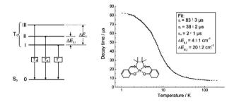
Fig. 5 Schematic energy-state diagram for the substates of the emitting  $T_1$  state of a transition metal complex (left). Plot of emission decay times of  ${\bf 16}$  in THF ( $\sim 10^{-5}$  M) versus temperature and the fit to the equation describing the temperature dependence of the measured decay time in a model of three substates (right) (adapted with permission from ref. 72. Copyright 2010, Wiley-VCH Verlag GmbH & Co. KGaA).
