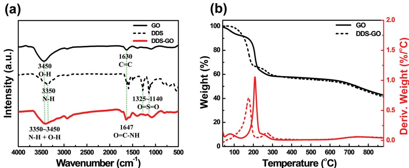
Fig. 2 (a) FT-IR spectra of GO, DDS, and DDS-GO. (b) TG-DTA curves of GO and DDS-GO during heating up to 900 °C under a N<sub>2</sub> atmosphere.
