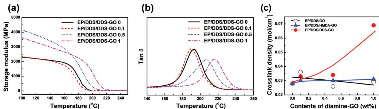
Fig. 7 DMA results of EP/DDS/diamine-GO nanocomposites. (a) Storage modulus, (b)  $\tan \delta$ , and (c) crosslink density of the EP/DDS/diamine-GO nanocomposites. Samples were tested in the temperature range of 30 to 260 °C at a scanning rate of  $3 \text{ °C min}^{-1}$ . The crosslink density was calculated using storage modulus and  $\tan \delta$  in the rubbery region of EP/DDS/diamine-GO nanocomposites.
