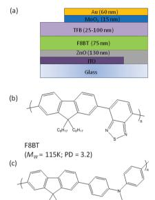
Fig. 3 (a) Schematic illustration showing the device architecture investigated and individual layer thicknesses, (b and c) molecular structures, molecular weight  $(M_w)$  and polydispersity (PD) information for F8BT and TFB.
