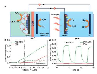
Fig. 6 (a) Schematic configuration of a PEC–MFC device; (b) I-V curves collected from a PEC device (red line) and a PEC–MFC device (olive line) with the Nb<sub>2</sub>O<sub>5-x</sub> NPs electrodes at a scan rate of 10 mV s<sup>-1</sup> with/without the white light illumination; (c) I-T curves recorded for the PEC device (red line) and the PEC–MFC device (olive line) at 0 V vs. Pt, with light on/off cycles.
