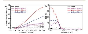
Fig. 4 (a) I-V curves measured under 100 mW cm<sup>-2</sup> simulated solar light generated by a 100 W xenon lamp coupled with an AM 1.5G filter in 1 M NaOH electrolyte; (b) IPCE spectra measured at 0.2 V vs. SCE in 1 M NaOH electrolyte.
