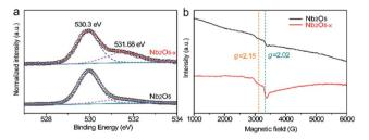
Fig. 2 (a) Normalized O 1s core-level XPS and (b) EPR spectra collected for Nb<sub>2</sub>O<sub>5</sub> and Nb<sub>2</sub>O<sub>5-x</sub> NPs films.
