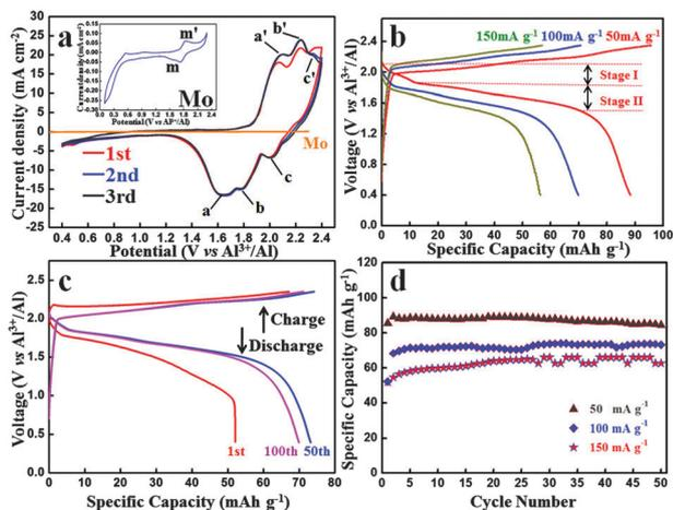
Fig. 2 (a) Cyclic voltammetry curve of an Al-ion full battery and that of Mo. The inset is the CV curve of Mo without carbon paper. (b) Charge and discharge curves under different current densities. (c) 1st, 50th and 100th charge–discharge curves at  $100 \text{ mA g}^{-1}$ . (d) Cycling performances of an Al-ion full battery under different current densities over 50 cycles.
