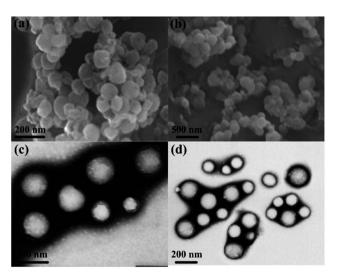
Fig. 1 SEM and TEM images of blank (a and c) and IBU-loaded (b and d) P(MMA3k-co-MAA4.5k)-b-PPEGMA5k assembled micelles.<sup>26</sup>
