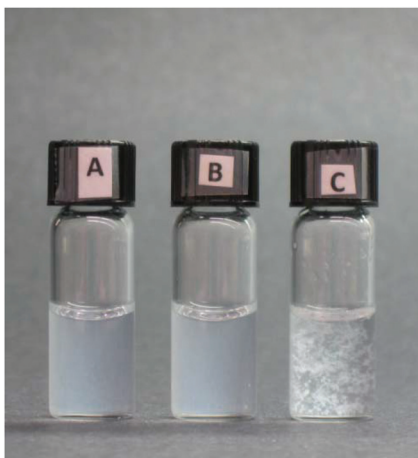
Fig. 2 Cross-linking of liposomes containing Zn 2 BDPA-PEG 2000 -DSPE and anionic target liposomes containing POPS. (A) Liposomes composed of Zn 2 BDPA-PEG 2000 -DSPE-cholesterol-POPC (2.5 : 30 : 67.5 mol%, 0.83 μmol total lipid) in zinc-containing HEPES buffer. (B) Liposomes composed of POPS-cholesterol-POPC (10 : 30 : 60 mol%, 0.83 μmol total lipid) in zinc-containing HEPES buffer. (C) Admixture of liposome samples A and B.
