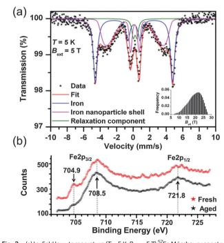
Fig. 2 (a) In-field low-temperature (T = 5 K,  $B_{\text{ext}} = 5 \text{ T}$ ) <sup>57</sup>Fe Mössbauer spectrum of the NZVI@FP nanocomposite. The solid-lines show the three components emerging from the deconvolution analysis. (b) Comparison of the XPS spectra recorded in the Fe2p region for the NZVI@FP nanocomposite freshly prepared (red pattern) and after ageing in air for one month (black pattern).
