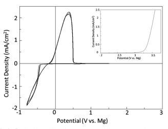
Fig. 1 Depicts the cyclic voltammogram and linear sweep voltammetry (insert) of 0.25 M MACC 2:1 solution in DME. The working electrode is Pt while the counter and reference electrodes are Mg metal. Measurements are obtained at 25 mV s<sup>-1</sup> and ambient conditions.
