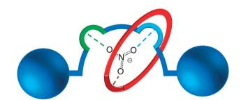
**Fig. 1** Schematic representation of a nitrate templated [2]rotaxane, with two hydrogen bonding recognition sites in the axle (blue and green) and one in the macrocycle (red), forming a complementary binding site for the trigonal nitrate anion between the interlocked components.
