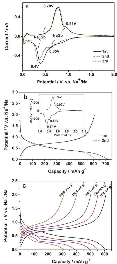
**Fig. 2** Electrochemical properties of the Sb/C nanocomposite: (a) The CV curve at a scan rate of 0.1 mV s<sup>-1</sup> (vs. Na<sup>+</sup>/Na); (b) charge–discharge curves of the Sb/C composite at a constant current of 100 mA g<sup>-1</sup>, the inset is differential capacity versus cell potential curve; (c) charge–discharge profiles at various current densities from 150 mA g<sup>-1</sup> to 2000 mA g<sup>-1</sup>.
