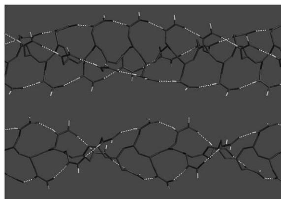
**Fig. 1** Possible conformations of tightly (top) and loosely (bottom) twisted helical *cis*-stereoregular poly(*N*-propargylamide) [–CH=C(CH<sub>2</sub>NHCOH)–]<sub>n</sub>, which accompany helically arranged intramolecular hydrogen-bonding strands (dotted lines) formed between the amide groups at the *i*<sup>th</sup> and (*i* + 3)<sup>th</sup> units (top) and the *i*<sup>th</sup> and (*i* + 2)<sup>th</sup> units (bottom). Methine and methylene hydrogen atoms are omitted for clarity.
