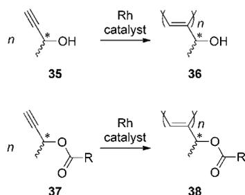
**Scheme 4** Polymerization of 1-methylpropargyl alcohols and esters.
