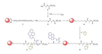
Scheme 1 Synthesis of (PyMMP-b-P2VP)-CdSe/ZnS QDs.
