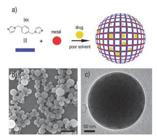
**Fig. 1** (a) Schematic illustration describing the encapsulation of drugs into metal–organic spheres created by the connection of metal ions, such as  $Zn^{2+}$ , through multitopic organic ligands, such as bix. (b) SEM and (c) TEM images of a representative colloidal solution of DOX/Zn(bix) spheres.
