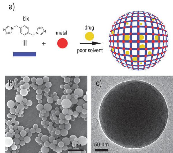
**Fig. 1** (a) Schematic illustration describing the encapsulation of drugs into metal–organic spheres created by the connection of metal ions, such as Zn<sup>2+</sup>, through multitopic organic ligands, such as bix. (b) SEM and (c) TEM images of a representative colloidal solution of DOX/Zn(bix) spheres.
