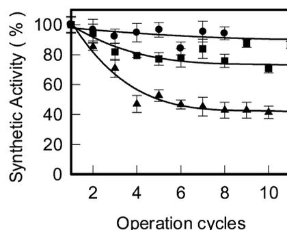
**Fig. 2** Deactivation profiles of *C. antarctica* lipase B in [BMIM][Tf<sub>2</sub>N] for continuous butyl butyrate synthesis in scCO<sub>2</sub> under different conditions (●, 40 °C and 15.0 MPa; ■, 50 °C and 12.5 MPa; ▲, 100 °C, 15.0 MPa).
