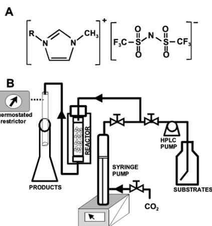
**Fig. 1** A. Structure of 1-alkyl-3-methylimidazolium triflimide, obtained according to Lozano *et al.*<sup>7</sup> B. Experimental set-up.
