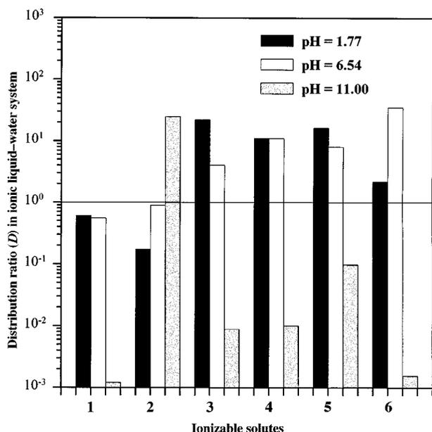
**Fig. 2** The solutes studied include: **1** phthalic acid ( $pK_1 = 2.89$ ,  $pK_2 = 5.51$ ), **2** aniline ( $pK_b = 9.42$ ), **3** 4-hydroxybenzoic acid ( $pK_1 = 4.48$ ,  $pK_2 = 9.32$ ), **4** benzoic acid ( $pK_a = 4.19$ ), **5** salicylic acid ( $pK_1 = 2.97$ ,  $pK_2 = 13.40$ ), **6** *p*-toluic acid ( $pK_1 = 2.27$ )
