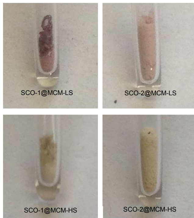
Fig. 1 Photographs showing the color change from LS (room temperature) to HS (~100 °C) for each sample.
