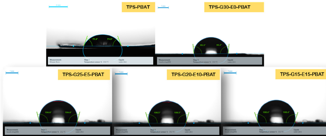
Fig. 4 Contact angle of the composite thin films.
