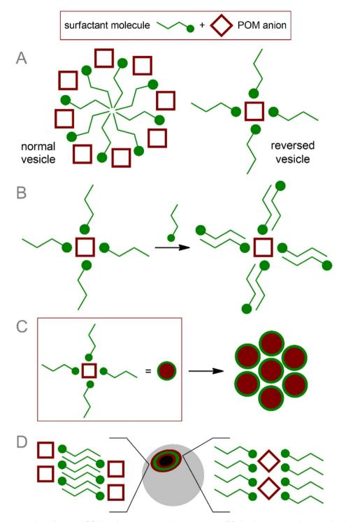
Fig. 1 Schematic representation of general POM-surfactant nanoparticle topologies: (A) simple normal and reversed vesicles; (B) concentric multilayer vesicles; (C) "blackberry"-type nanoparticles; (D) hollow membrane normal and reversed vesicles.
