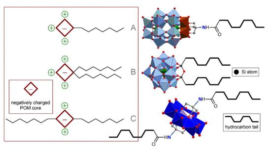
Fig. 2 Schematic representation and archetype examples of POM-based surfactants: (A) POM head-hydrophobic tail; (B) POM head-several hydrophobic tails; (C) tail-POM head-tail.
