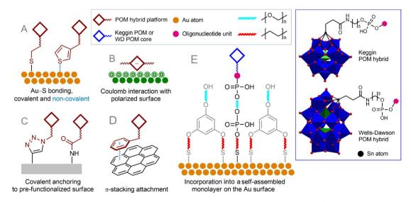
Fig. 8 Organo-functionalized POMs tethered on the surfaces with covalent or non-covalent interaction (A-D). Incorporation of monoligated POMs into a self-assembled monolayer on the Au surface (E).
