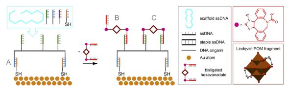
Fig. 11 DNA origami structure assembly involving POM-ssDNA building blocks. The preformed DNA origami structure immobilized on Au(111) through thiol groups (A) and conjugated to Lindqvist-type hexavanadate units augmented with ssDNA fragments by pairing complementary nucleotide sequences (B and C).
