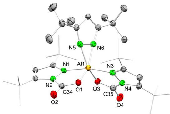
**Fig. 4** Crystal structure of Al(CO<sub>2</sub>·pz<sup>tBu</sup>)<sub>2</sub>(pz<sup>tBu</sup>) (**1-CO<sub>2</sub>**). Ellipsoids are set at the 50% probability level. Hydrogen atoms and disorder in the *t*Bu moieties are omitted for clarity. See ESI† for selected interatomic distances and angles.
