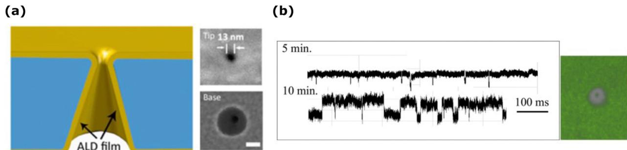
**Fig. 8** (a) Schematic illustration of uniform ALD coating on a single conical nanochannel and SEM images of the tip and base sides. The scale bar is 100 nm. Reprinted with permission from ref. 279 Copyright 2015, American Chemical Society. (b) (Left) Resistive pulse signals of a 1 : 1 mixture of 22 b ss-DNA and ds-DNA after 5 min and 10 min. (Right) STED super-resolution microscopy image at 30 min. Reprinted from ref. 280 with the permission of AIP Publishing.
