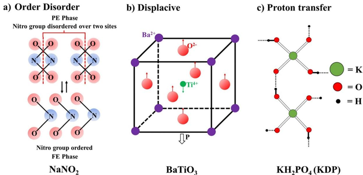
Fig. 5 Different types of mechanisms that lead to the origin of ferroelectricity polarization.
