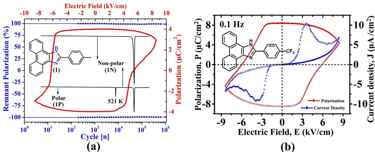
Fig. 9 (a) Depiction of ferroelectricity, thermal stability and phase transition behaviour in 2-(*p*-tolyl)-1*H*-phenanthro[9,10-*d*]imidazole.<sup>54</sup> (b) Ferroelectric loop ( $P$  vs.  $E$ ) and the corresponding fatigue measurements in 2-(4-(trifluoromethyl)phenyl)-1*H*-phenanthro[9,10-*d*]imidazole.<sup>61</sup>
