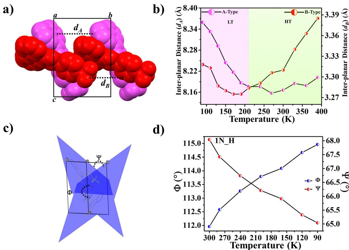
Fig. 17 For 1P\_O (Fig. 4), (a) stacking of molecules A (pink) and B (red) along [010] and (b) variation of inter-planar distances  $d_A$  and  $d_B$  with temperature. For 1N\_H (Fig. 4), (c) dihedral angles  $\Phi$  and  $\Psi$  between the molecular planes passing through the adjacent molecules A and B, forming an open bookcase-like geometry while viewing down [110] and (d) the variation of  $\Phi$  and  $\Psi$  with temperature.<sup>61</sup>
