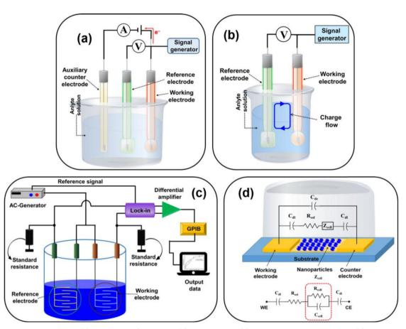
Fig. 10 Representing the diagram of (a) amperometric/voltametric, (b) potentiometric, (c) conductometric biosensors, and (d) equivalent circuit of the impedometric biosensor. [Reproduced from ref. 157 with permission from [MDPI], copyright [2021]]
