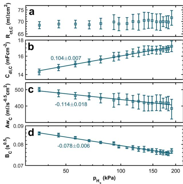
Fig. 7 Double-logarithmic plots of (a) the cathodic charge transfer resistance; (b) the double layer capacitance  $C_{dl,C}$ ; (c) the first Warburg short parameter  $Aw_C$ ; and (d) the second Warburg short parameter  $B_C$  vs.  $p_{H_2}$ .
