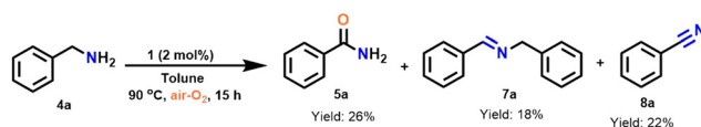
Scheme 2 1-Catalysed aerial oxidation of benzylamine ( 4a ) in the absence of a base.
