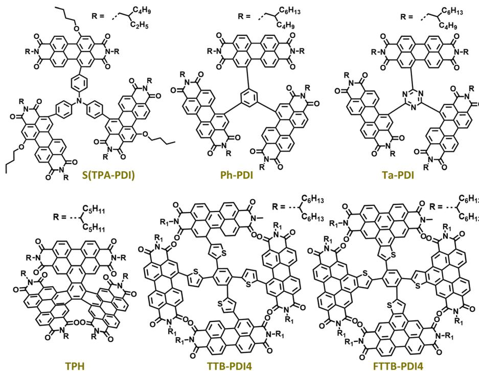
Fig. 6 Representative structures of PDI-based multimer acceptors.
