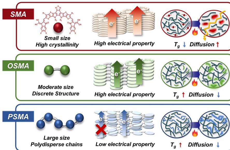
Fig. 1 Comparison in molecular configuration, electrical properties, and diffusion characteristics of SMAs, OSMA, and PSMA.
