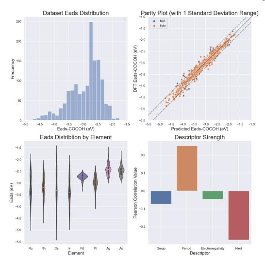
Fig. 4 (a) Adsorption energy distribution of the entire \*COCOH dataset, (b) parity plot with dotted lines outlining 1 standard deviation error, (c) adsorption energy distribution by element Cu is alloyed with, (d) Pearson correlation value of each descriptor averaged across all 13 nearest atoms to the adsorbate
