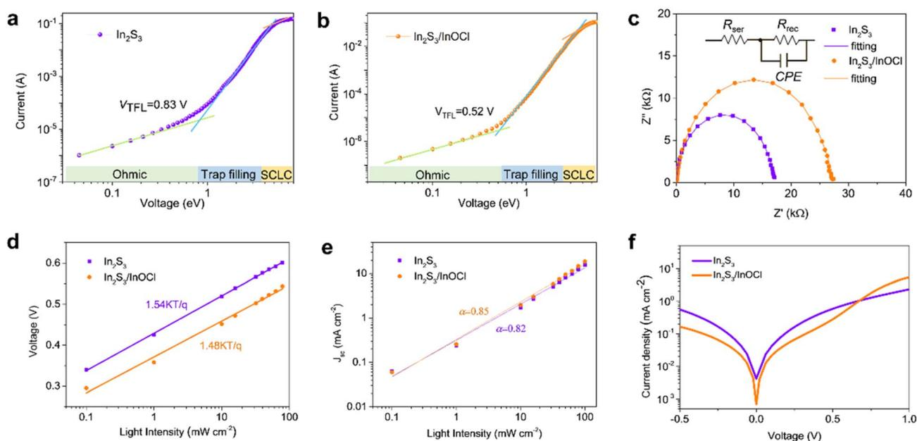
**Fig. 5** (a and b) The SCLC measurements of  $\text{In}_2\text{S}_3$  and  $\text{In}_2\text{S}_3/\text{InOCl}$ -based electron-only single-carrier devices, and (c) the impedance spectroscopy spectra, (d) light intensity-dependent  $V_{oc}$  measurements, (e) light intensity-dependent  $J_{sc}$  measurements, and (f) dark  $J$ - $V$  curves of  $\text{In}_2\text{S}_3$  and  $\text{In}_2\text{S}_3/\text{InOCl}$ -based  $\text{Sb}_2(\text{S,Se})_3$  solar cells.
