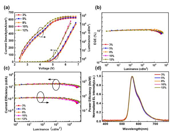
Fig. 2 EL performance of yellow OLEDs with the doping concentrations of 3%, 5%, 8%, 10%, and 12% for the PO-01 materials. (a) Current densityvoltage-luminance curves. (b) EQE-luminance curves. (c) Current efficiency-luminance-power efficiency curves. (d) EL spectra at a voltage of 4 V.
