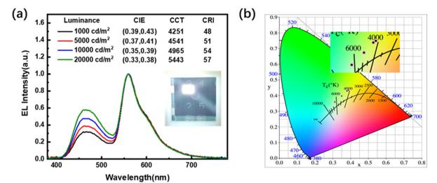
(a) EL spectra and color coordinates (b) of device W3 at different luminance values.
