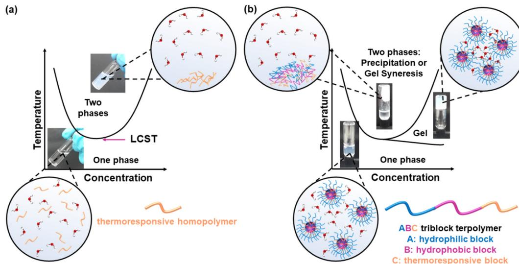
**Fig. 1** Phase diagrams of (a) an aqueous solution of a thermoresponsive homopolymer presenting LCST behaviour and (b) an aqueous solution of a thermoresponsive ABC triblock terpolymer with LCST type thermogelling behaviour; A, B, and C blocks are shown in blue, purple, and orange, respectively.
