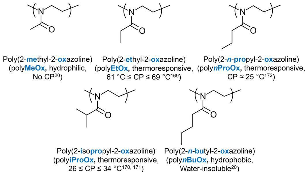
Fig. 11 Chemical structures and properties of poly(2-oxazoline)s.
