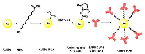
Fig. 2 Schematic presentation of the conjugation of the mAb on the surface of MUA-modified AuNPs. Reprinted from ref. 23. E. Karakuş et al., Anal. Chim. Acta, 2021, 1182, 338939-338949. Copyright (2021) Elsevier.
