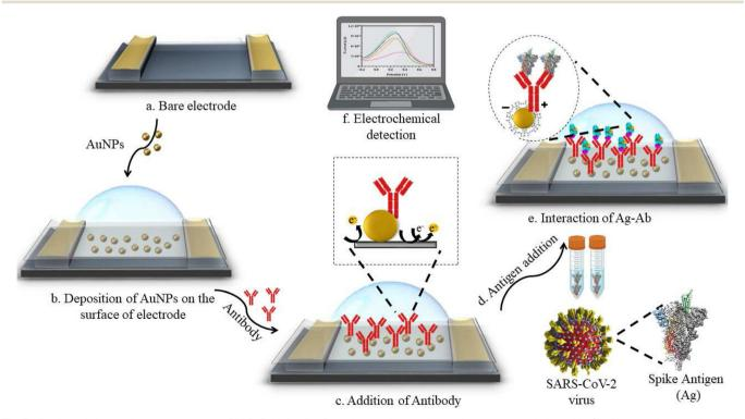
Fig. 3 Design of electrochemical sensing of SARS-CoV-2 spike S1 antigen using an electrode system consisting of Aq/AgCl as a reference electrode and platinum as a counter electrode. Reprinted from ref. 34. A. Robert et al., Anal. Chim. Acta, 2021, 1188, 339207-339219. Copyright (2021) Elsevier.
