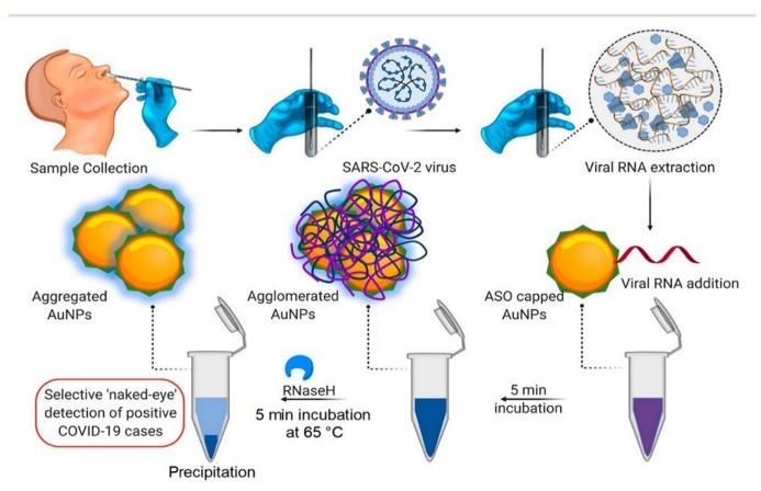
Fig. 4 Schematic representation for the naked-eye detection of SARS-CoV-2 RNA mediated by the suitably designed ASO-capped AuNPs. Reprinted from ref. 47. P. Moitra et al., ACS Nano, 2020, 14, 7617-7627. Creative Commons public use license.
