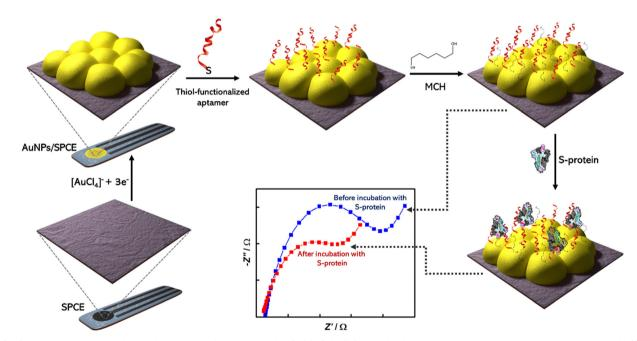
Fig. 9 Schematic representation of fabrication of aptasensor for SARS-CoV-2 S-protein detection using screen printed carbon electrode (SPCE); Reprinted from ref. 62; Abrego-Martinez et al., Biosen. Bioelectron., 2022, 113595. Copyright (2022) Elsevier.
