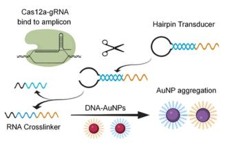
Fig. 6 Schematic representation of the principle of Cas-mediated AuNP aggregation and corresponding change in color from red to purple. Reproduced from ref. 53. Y. Cao et al., Chem. Comm., 2021, 57, 6871-6876. Copyright (2021) Royal Society of Chemistry.
