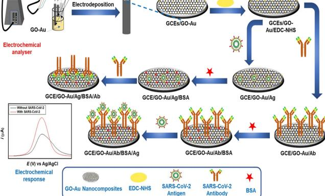
Fig. 8 Schematic of steps involved in the fabrication of SARS-CoV-2 antigen and SARS-CoV-2 antibody immunosensors. Reprinted from ref. 57. M. A. Sadique et al., ACS Appl. Bio Mater., 2022, 5, 2421-2430. Copyright (2021) Creative Commons public use license.
