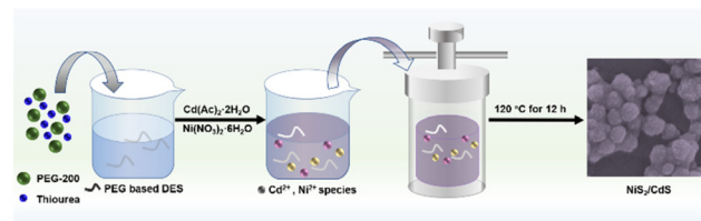
Fig. 1 A schematic illustration of the formation of \text{NiS}_2/\text{CdS} photocatalyst.
