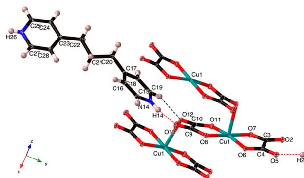
Fig. 4 The asymmetric unit of C<sub>13</sub>H<sub>16</sub>N<sub>2</sub>[Cu(C<sub>2</sub>O<sub>4</sub>)<sub>2</sub>] (**2**) with one extra oxalate, one extra Cu and one additional N–H. The Cu–O7 is 2.538 Å, which is normal for an axial Jahn–Teller bond.
