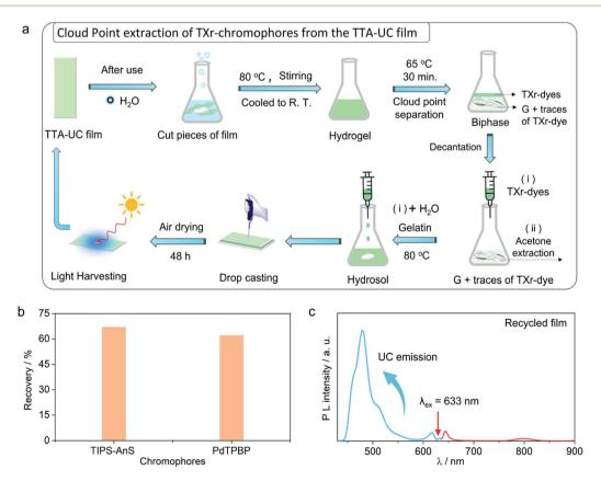
Fig. 5 Circular use of key bioplastics components. (a) Illustration of the recycling of G-TXr-TIPS-AnS-PdTPBP film. (b) Plot showing % recovery of chromophores and (c) UC emission spectrum of the recycled film upon 633 nm laser excitation ( $I_{\rm ex}=1.3~{\rm W~cm}^{-2}$ ).
