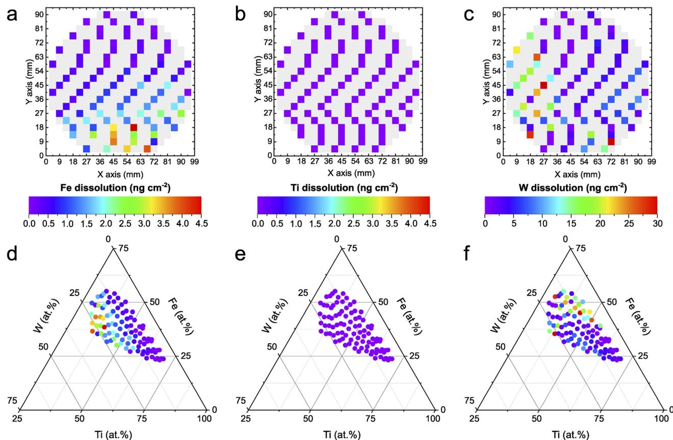
Fig. 2 Element-specific dissolution of Fe–Ti–W–O material library at 1.7  $V_{\text{RHE}}$ . (a–c) Dissolved amounts of Fe (a), Ti (b), and W (c) mapped onto a schematic representation of the wafer. (d–f) Dissolved amounts of Fe (d), Ti (e), and W (f) mapped onto a ternary diagram. The HT measurements were conducted in 0.05 M  $\text{NaNO}_3$  (pH 5.7) under 1 Sun Am 1.5G illumination. Note that the color scale for W differs from Fe and Ti.
