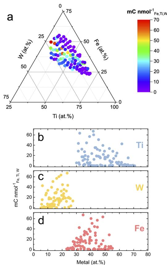
Fig. 3 Photocharge normalized by the total dissolution of the Fe–Ti–W–O material library measured at 1.7 V<sub>RHE</sub>. (a) Dissolution-normalized photocharge mapped onto a ternary diagram. The performance metric is further plotted over the specific Ti (b), W (c), and Fe (d) content in the oxide films.
