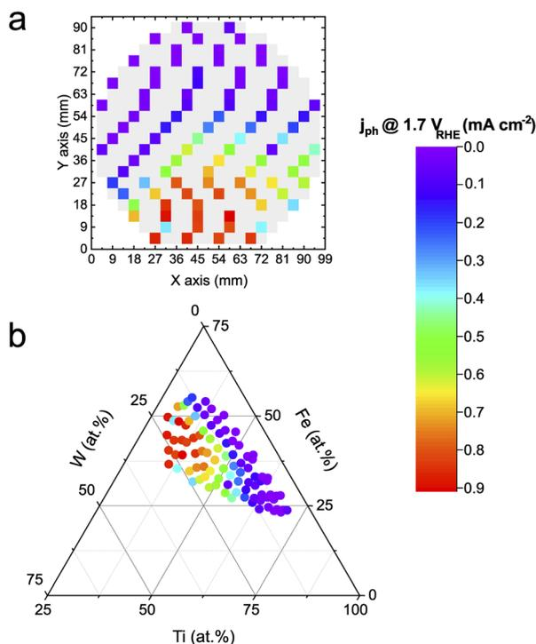
Fig. 1 Photocurrent densities of Fe–Ti–W–O material library at 1.7 V<sub>RHE</sub>. (a) Photocurrent density mapped onto a schematic representation of the wafer. (b) Photocurrent density mapped onto a ternary composition diagram of the metal constituents. The HT measurements were conducted in 0.05 M NaNO<sub>3</sub> (pH 5.7) under 1 Sun Am 1.5G illumination.
