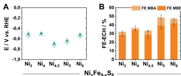
Fig. 2 Half-cell potentials of the herein investigated  $\text{Ni}_x$  pellet electrodes after 2 h of electrolysis at  $100 \text{ mA cm}^{-2}$  (A). The respective faradaic efficiency values *via* GC-MS quantification (B).
