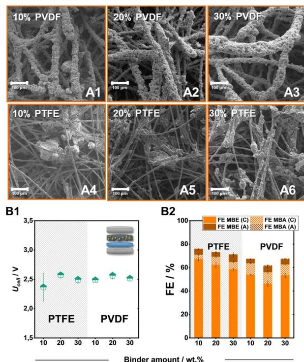
Fig. 4 Scanning electron microscopy (SEM) investigation of PVDF (A1–A3) and PTFE bound electrodes (A4–A6). Effect of the binder nature and content on the ECH of MBY at 80 mA cm<sup>-2</sup>. The obtained cell voltage (B1) and faradaic efficiency (B2). Here, FE<sub>MBX</sub> (C) and FE<sub>MBX</sub> (A) (X: E, A) correspond to the FE values of ECH products detected in the catholyte and anolyte after electrolysis, respectively.
