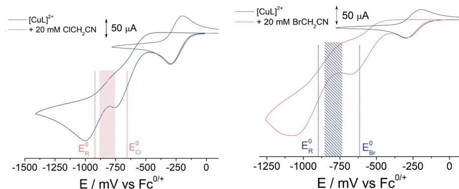
Fig. 1 CV of  $[Cu^{II}L(NCCH_3)]^{2+}$  (2 mM) before and after the addition of 10 equivalents (20 mM)  $ClCH_2CN$  (left, **1a**) and  $BrCH_2CN$  (right, **1b**) (at a scan rate of  $100 \text{ mV s}^{-1}$ ; highlighted shaded areas show the potential window for forming  $[Cu^{II}L(CH_2CN)]^+$ ).
