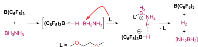
Scheme 59 Mechanistic proposal for the dehydrocoupling of NH_3 \cdot BH_3 .
