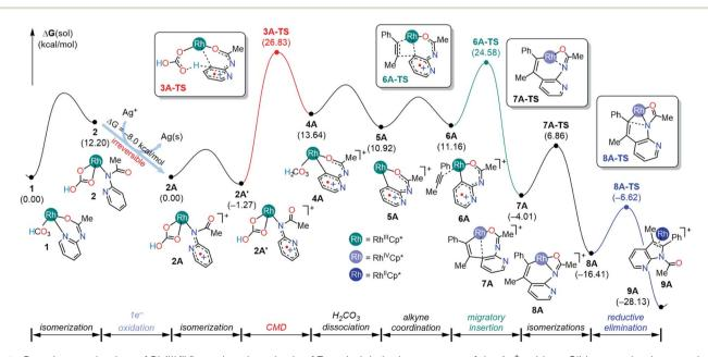
Fig. 4 Reaction mechanism of Rh(III/IV)-catalyzed synthesis of 7-azaindole in the presence of the  $Ag^+$  oxidant. Gibbs energies, in parenthesis, are in kcal  $mol^{-1}$ .
