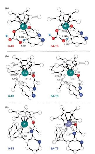
Fig. 5 Selective illustrations for the comparison of the transition state of (a) CMD, (b) migratory insertion, and (c) reductive elimination in the neutral and cationic pathways. Bond lengths have the units of Angstrom (Å). Nonessential hydrogen atoms are omitted for clarity.
