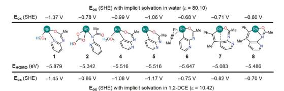
Fig. 2 Computed oxidation potentials and HOMO energies of Rh(III) complexes.
