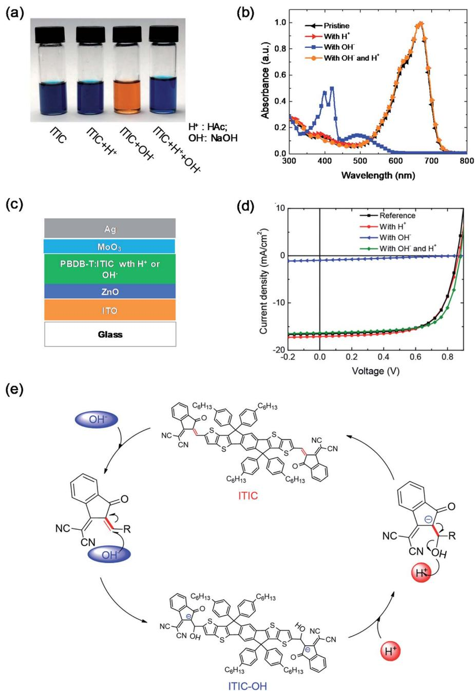
Fig. 5 (a) Image, and (b) the absorbance of four different ITIC solutions: pristine, and with the addition of  $\text{H}^+$ ,  $\text{OH}^-$ , and both  $\text{OH}^-$  and  $\text{H}^+$ ; (c) device structure; (d)  $J$ - $V$  characteristics of devices with active layers having acid or base additives; (e) scheme of the reversible reaction of ITIC under acidic and basic conditions. Reproduced from ref. 44 with permission from the American Chemical Society, copyright [2019].
