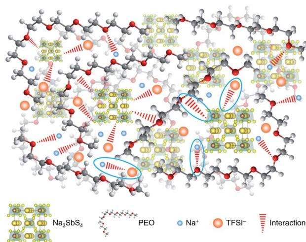
Fig. 4 Schematic diagram of the structure of the PEO/NaTFSI/Na<sub>3</sub>SbS<sub>4</sub> electrolyte, where the four types of interactions between the different components (Na<sub>3</sub>SbS<sub>4</sub> and TFSI<sup>-</sup>, Na<sub>3</sub>SbS<sub>4</sub> and PEO, Na<sup>+</sup> and PEO, Na<sup>+</sup> and TFSI<sup>-</sup>) are highlighted.
