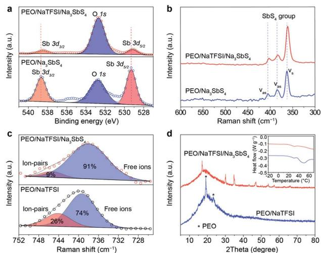
Fig. 3 Interactions between components in the PEO-based all-solid-state electrolytes. (a) Sb 3d XPS spectra and (b) Raman spectra of the PEO/Na<sub>3</sub>SbS<sub>4</sub> and PEO/NaTFSI/Na<sub>3</sub>SbS<sub>4</sub> electrolyte. (c) Raman spectra and (d) XRD patterns of the PEO/NaTFSI electrolyte and PEO/NaTFSI/Na<sub>3</sub>SbS<sub>4</sub> electrolyte. Inset: corresponding DSC curves.
