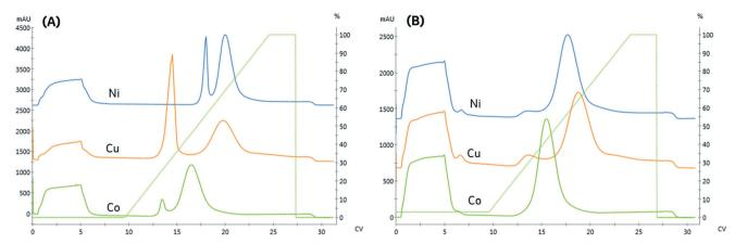
Fig. 3 Comparing the binding and elution profiles when the IDA resin is charged with different divalent metals (nickel, copper, and cobalt). A fixed linear gradient,  $\gamma = 11.3$  was employed for trials where: (A) no imidazole is included in the sample or pre-elution wash (B) 15 mM imidazole is included in the sample and pre-elution wash.
