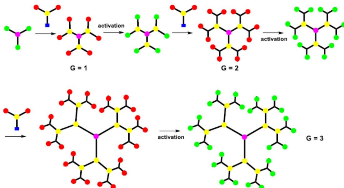
Fig. 3 Structure of dendrimers in divergent approach method.
