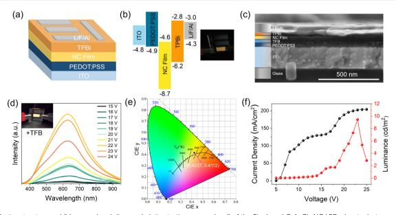
Fig. 5 (a) Device structure and (b) energy band diagram (relative to the vacuum level) of the Sb-doped CsAqCl<sub>2</sub> NC LEDs. Inset: photograph of an LED driven by a 14 V bias. (c) Cross-sectional SEM image of a TFB-incorporated device. (d) EL spectra of the resulting LEDs at different applied voltages. Inset: photograph of the LED driven by a 22 V bias. (e) CIE coordinates and (f) I-V-L characteristics of the LED devices.
