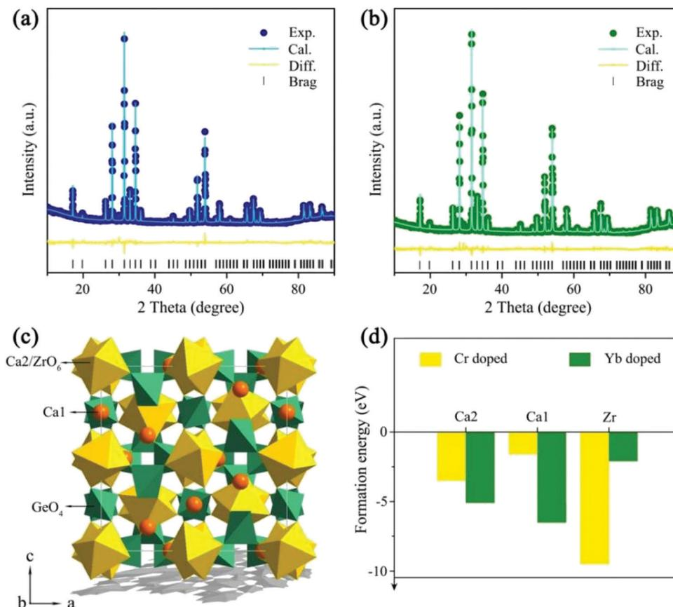
Fig. 1 Powder XRD Rietveld refinements of (a) blank CZGO and (b) CZGO: 1% Cr<sup>3+</sup>, 1% Yb<sup>3+</sup>; (c) the crystalline structure and cationic sites in CZGO; (d) the formation energy of Cr or Yb doped into the different cationic sites Ca1O<sub>8</sub>, Ca2/ZrO<sub>6</sub>, and GeO<sub>4</sub>.
