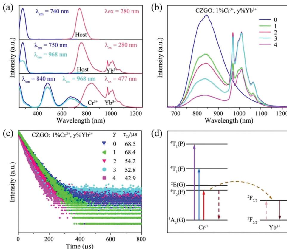
Fig. 6 (a) The PL and PLE spectra of the blank, and Yb<sup>3+</sup>-doped and Cr<sup>3+</sup>/Yb<sup>3+</sup>-co-doped CZGO; (b) PL spectra and (c) decay curves of CZGO: 1% Cr<sup>3+</sup>, y% Yb<sup>3+</sup> (y = 0, 1, 2, 3, 4) excited by 480 nm light together with (d) an energy transfer schematic diagram between Cr<sup>3+</sup> and Yb<sup>3+</sup>.
