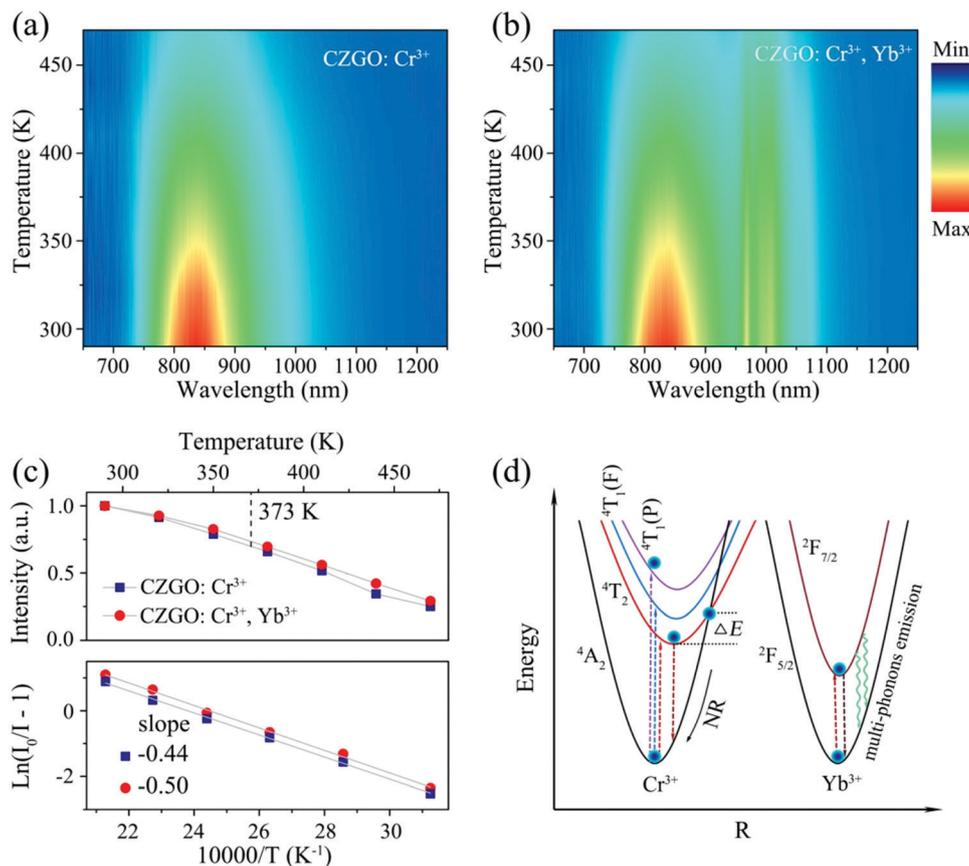
Fig. 7 The temperature-dependent PL spectra of (a) 1% Cr<sup>3+</sup> and (b) 1% Cr<sup>3+</sup>/1% Yb<sup>3+</sup> co-doped CZGO; (c) normalized integrated intensity and a plot of  $\ln(I_0/I - 1)$  vs.  $10\,000/T$  for Cr<sup>3+</sup> and Cr<sup>3+</sup>/Yb<sup>3+</sup> co-doped CZGO; (d) a configuration coordinate diagram for Cr<sup>3+</sup> and Yb<sup>3+</sup> in the CZGO host.
